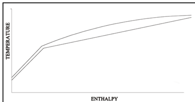
Figure 3. Typical composite cooling and warming curves for double nitrogen expander cycle.
